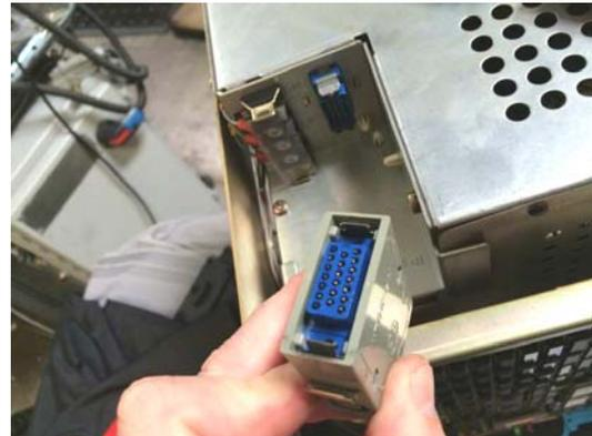
4. Unscrew the three CRT power wires from the terminal block, and cover the three ring terminals with heat-shrink tubing or electrical tape to keep them from shorting to anything later, because they are 220 volts AC.
