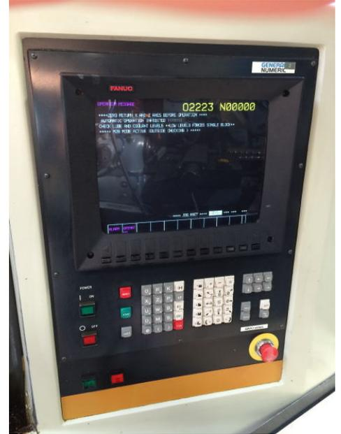
12. After the display and bezel were mounted, we had to adjust the XVGA Box settings so that the image was correctly sized and positioned behind the original bezel and above the correct soft-keys:
